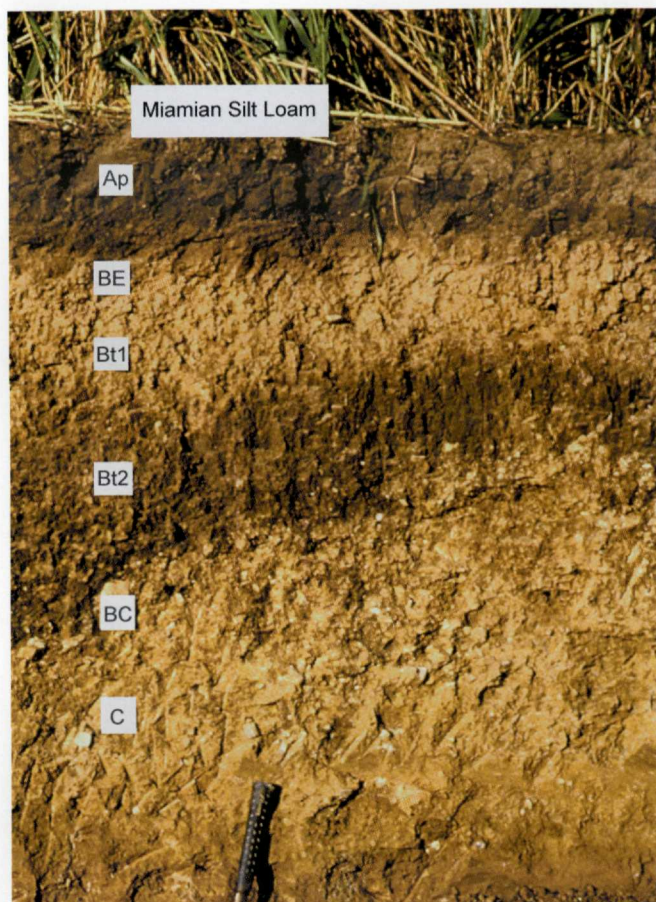
FIGURE 1. Miamiian soil profile at the Molly Caren Agricultural Center near London, OH. Soil horizons are distinguished by particular assemblages of morphological properties: color, texture, structure, consistence, and soil reaction.
