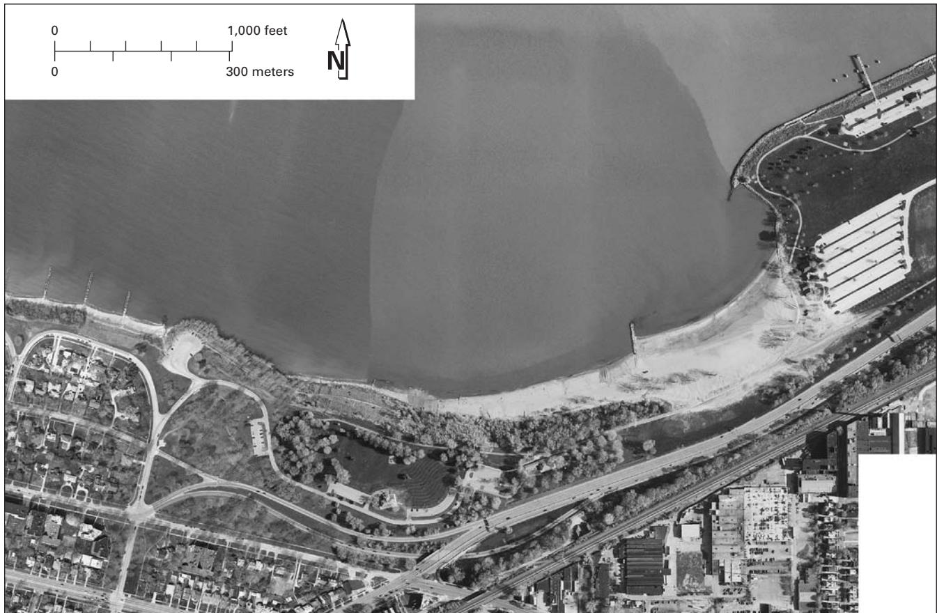
FIGURE 31.—Beach sand at Edgewater Park in Cleveland, Ohio, is trapped by a bulkhead and a groin. Note wind-blown sand near the Shoreway and southwest of the parking lot. The eastern part of the park, shoreward of the stone bulkhead, is all filled land. An oval parking lot at the western end of the park sets atop a small headland composed of Chagrin Shale. West of the headland, groins at Perkins Beach have deteriorated and no longer trap much sand. Aerial photograph taken in 2002 by the Cuyahoga County Engineer.
