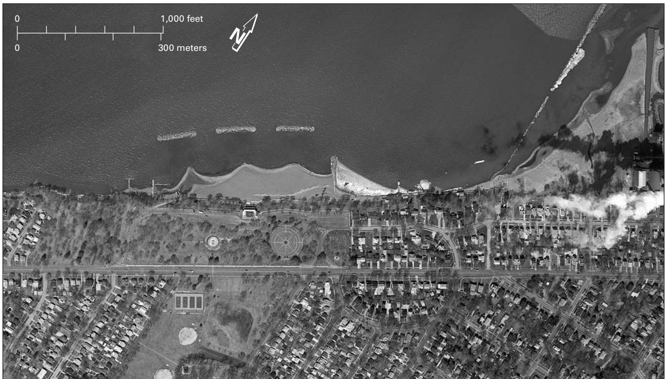
FIGURE 35.—Lorain Harbor and Lakeview Park in Lorain, Ohio, in 1999. The segmented breakwaters are designed to form salients rather than a tombolos. Compare size and shape of beaches at the park and inside harbor with beaches in 1973 (fig. 34). Aerial photograph taken by the Lorain County Auditor.
