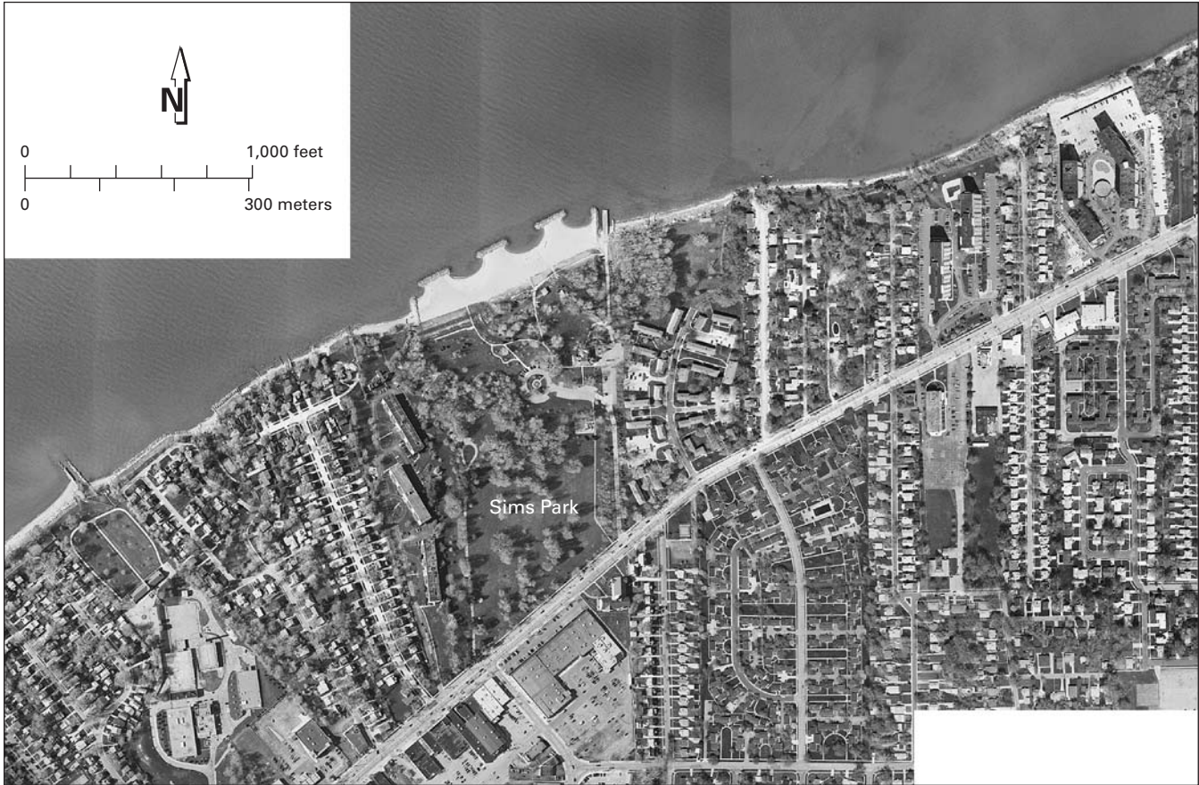
FIGURE 26.—Sims Park in Euclid, Ohio, is located on a broad headland of Devonian shale. Shale crops out in the lower part of the bluff along the western half of the photo but drops below lake level in the eastern part of the photograph. Even though shale is more resistant to erosion than the till found to the east, much of the shale headland is now armored to prevent erosion. To the east, large amounts of fill have been dumped over the bluff edge to reclaim land lost to erosion and to protect the shore. Aerial photograph taken in 2002 by the Cuyahoga County Engineer.
