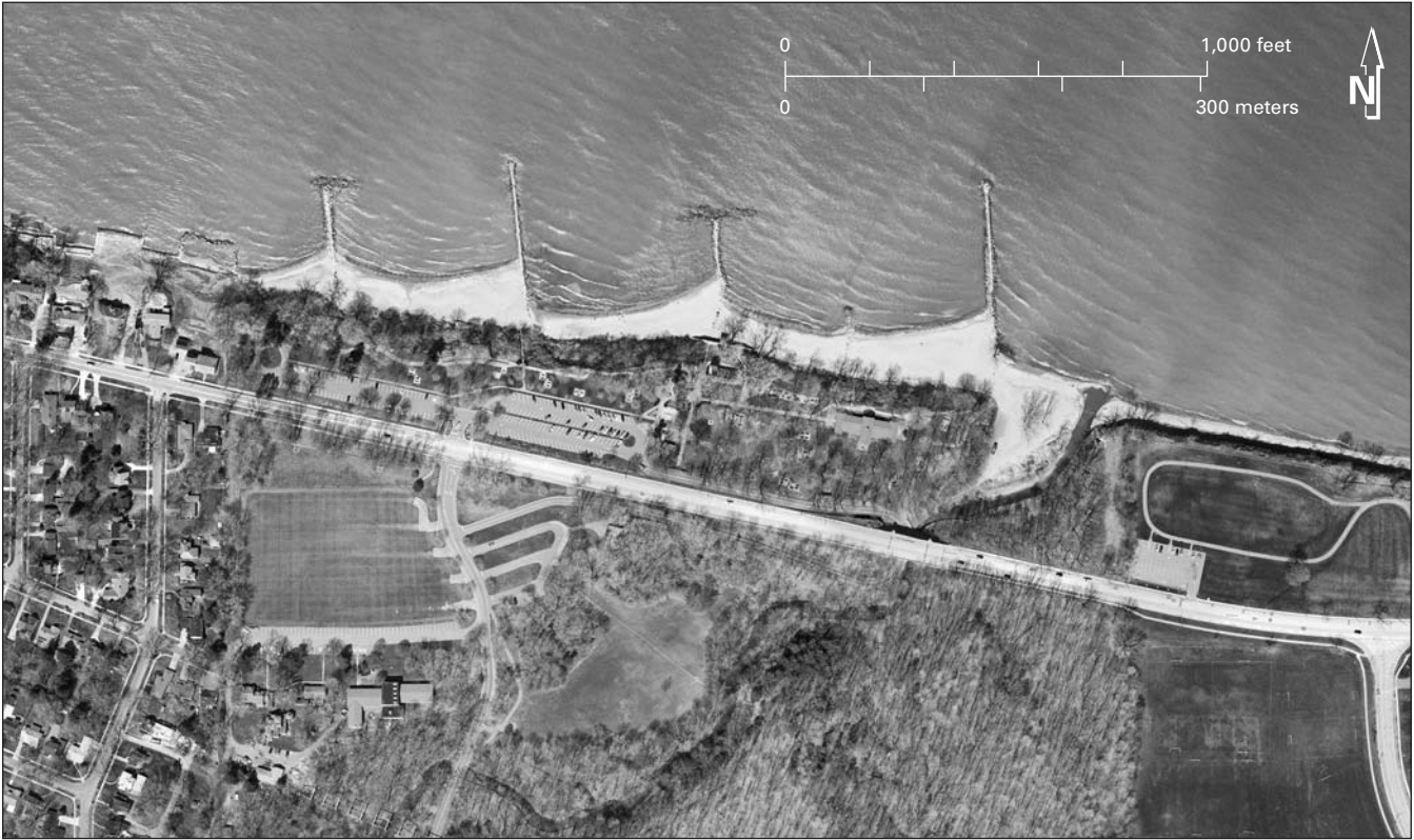
FIGURE 32.—Huntington Reservation in Bay Village, Ohio. Sandstone block groins trap sand to form beach. West of the park, a variety of structures protect the slope of till, glaciolacustrine sediment, and fill. East of the park, the shale cliff is unprotected. Aerial photograph taken in 2002 by the Cuyahoga County Engineer.
