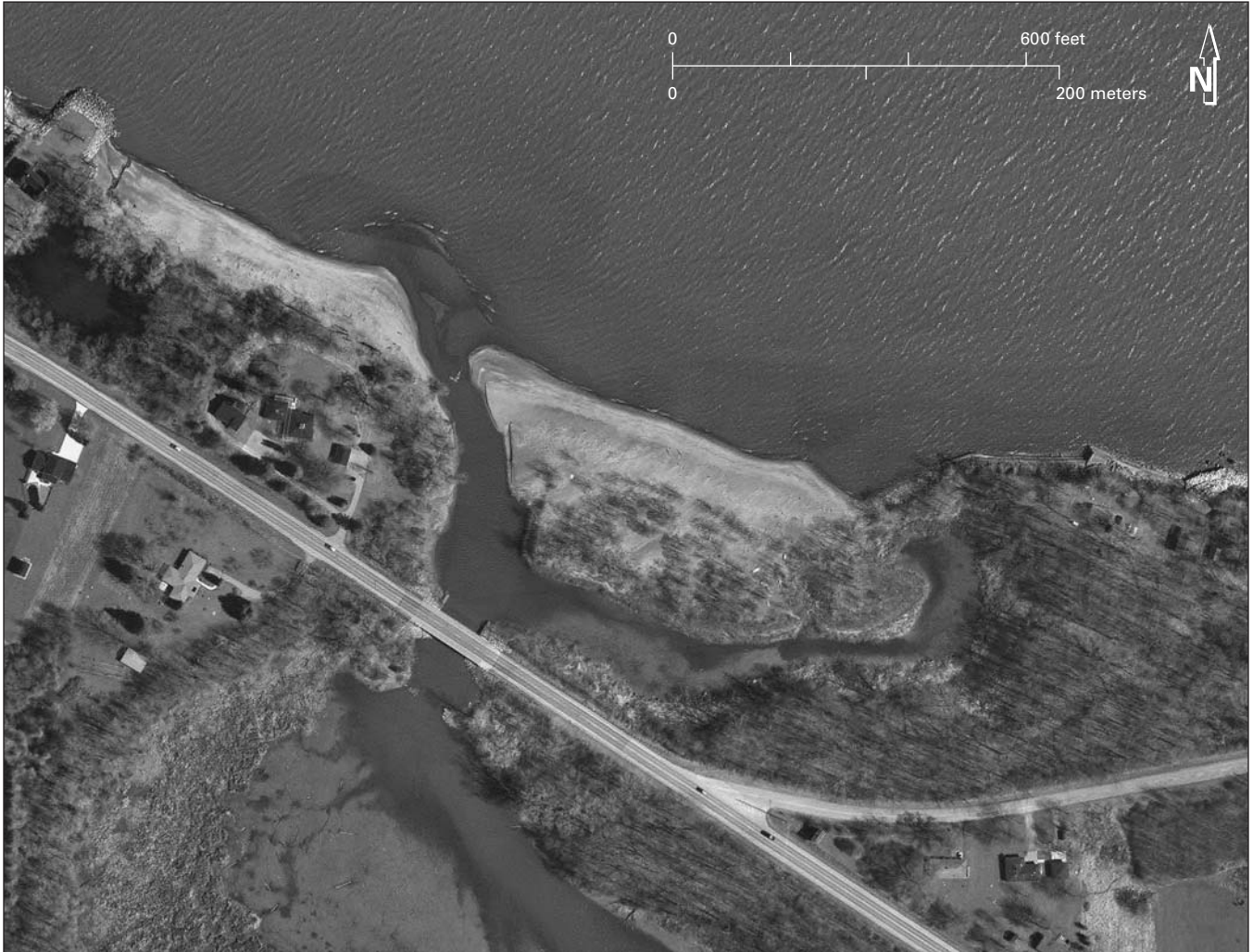
FIGURE 40.—Old Woman Creek in Huron, Ohio. The abandoned stream channel from the 1970s appears on the east side of the floodplain. Westward displacement of the stream mouth suggests a net east-to-west transport of sand along this reach of shore. Aerial photograph taken in 2003 by the Erie County Auditor.
