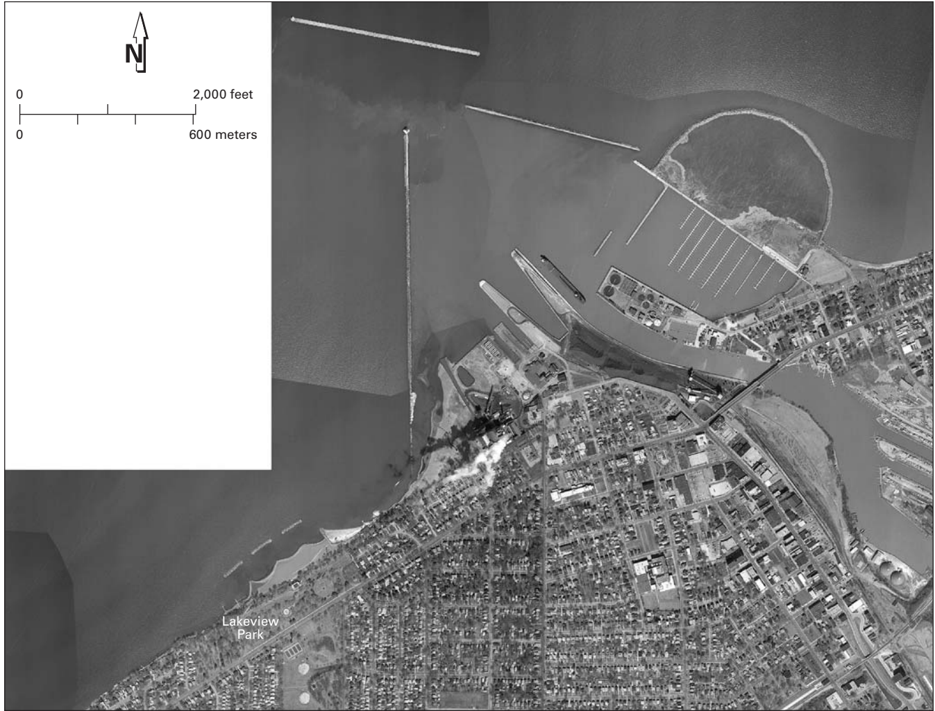
FIGURE 33.—Lorain Harbor and Lakeview Park in Lorain, Ohio. The confined disposal facility (CDF) attached to the east breakwater is nearly filled. Note sand in southwest corner of harbor. Aerial photograph taken in 1999 by the Lorain County Auditor.
