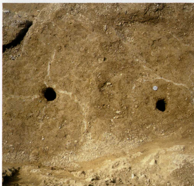
FIGURE 2. Photograph showing the 50 mm diameter boreholes used for hydraulic conductivity tests. Note the coin (the quarter above and to the left of the right hole) used for scale, and the size and arrangement of the fracture-affected zones relative to the boreholes.
