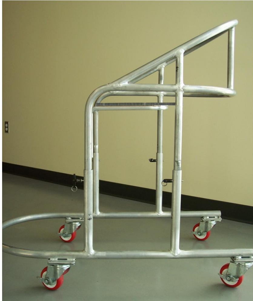
Figure 31: The Completed Frame of the New Walker.
