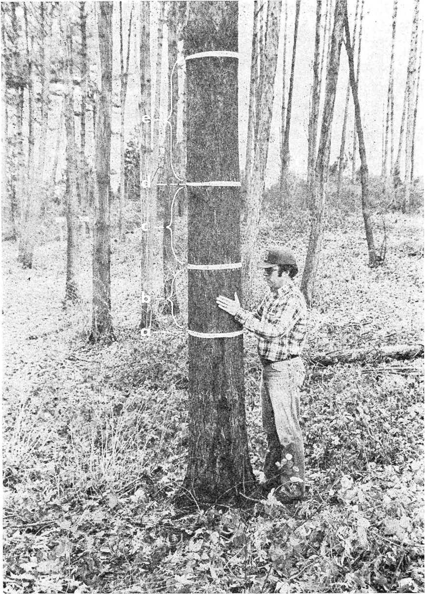
FIG. 1. —Illustration of points on white pine stem used in estimating site index based on 3-, 5-, or 10-year growth intercept measurements: a = base of breast high (BH) annual height increment, b = BH annual height increment, c = first annual height increment above BH increment, d = base of second annual height increment above BH increment, and e = second annual height increment above BH increment.
