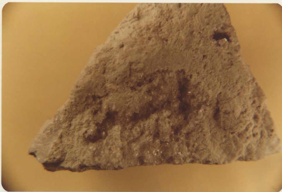
Photograph of quartz on rhyolite typical of the area. Specimen is 2 inches in length.
