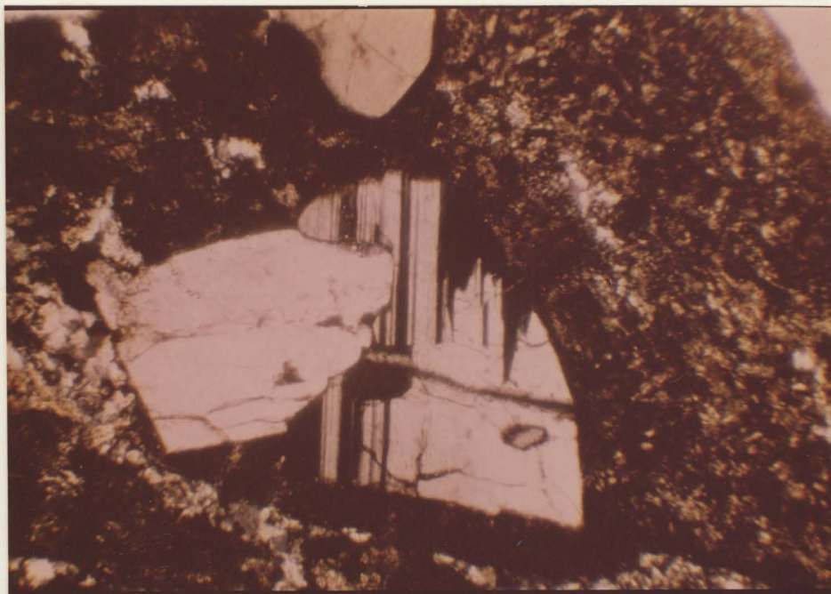
Photomicrograph of plagioclase. Crossed nicols, 40X. From slide 2.
