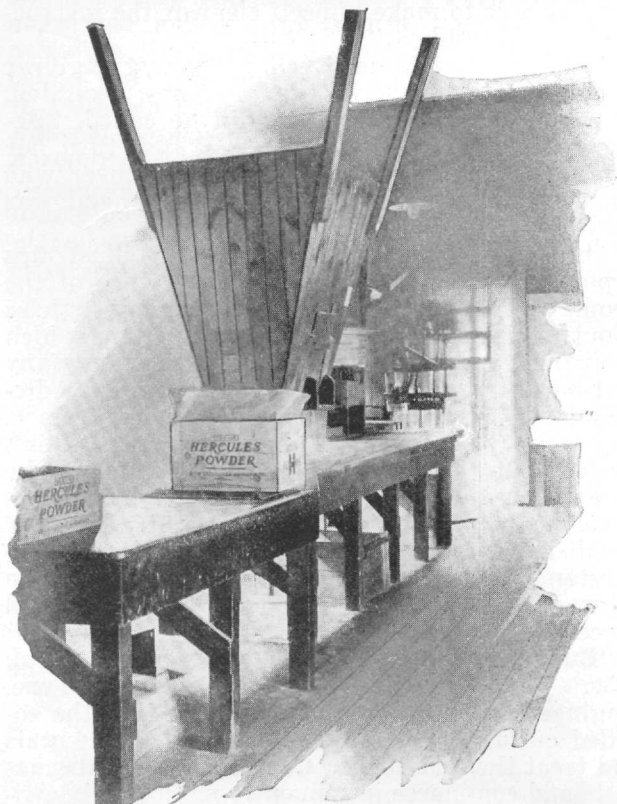
The Filled Cartridges Are Placed in Wooden Boxes Lined with Paraffin Paper at the Box Packing House
