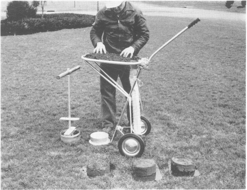
Fig. 1.—The 1/3-square-foot sampler, portable table, and size of cores removed for examination.
