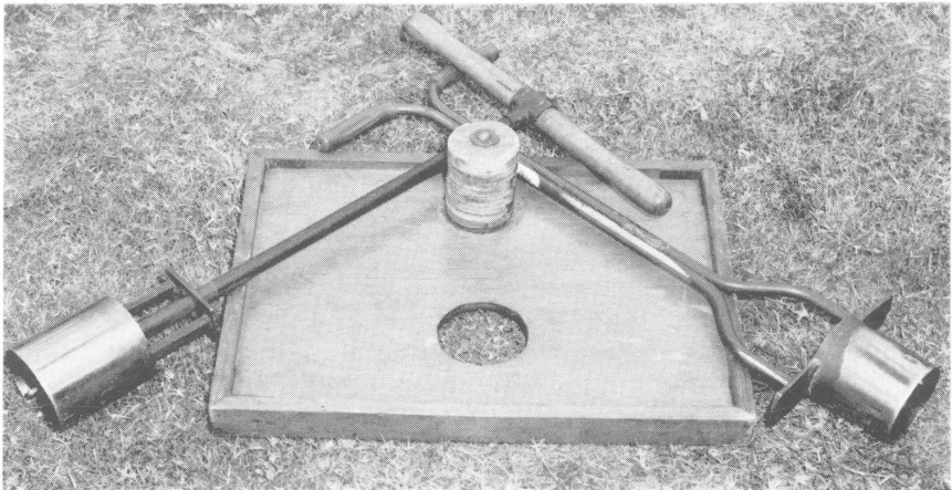
Fig. 2.—1/12-square-foot samplers and the board used in examining soil for Japanese beetle larvae.
