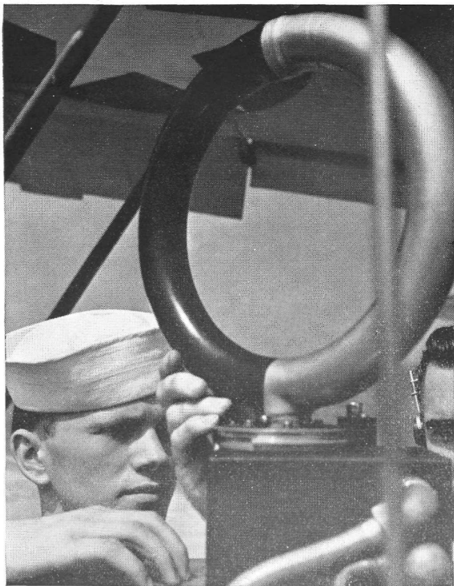
• Using a loop antenna for direction finding by discovering the null point.
