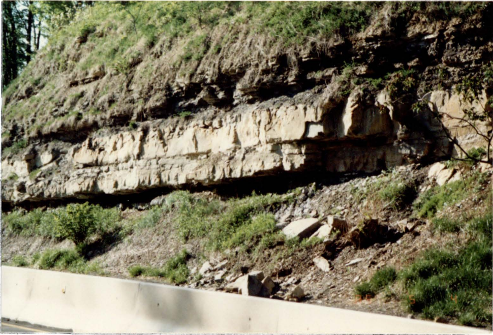
Photo 5. Coarse grained, micaceous sandstone exposed along Route 40, 5 miles west of Brownsville, Pennsylvania.
