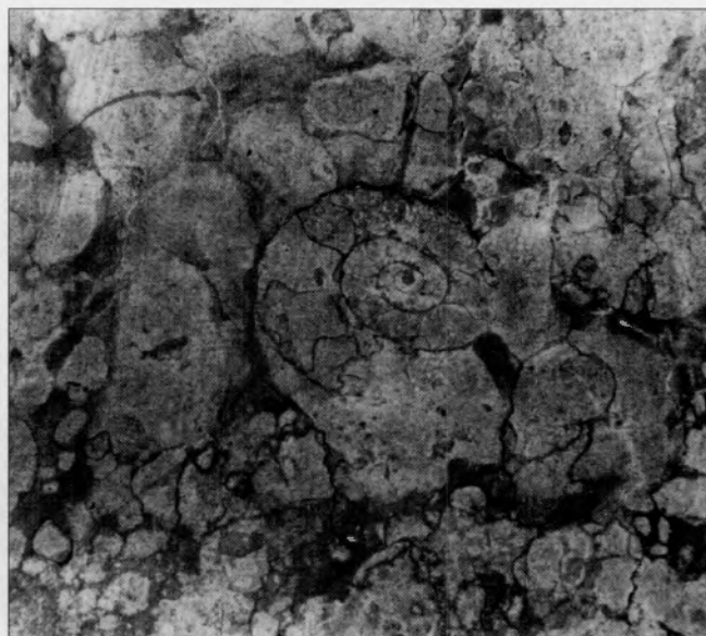
FIGURE 39.—Close-up of Verona marble in the entranceway of Union Terminal (Museum Center). The fossil in the center of the photograph is an ammonite, seen in an oblique cross section, and is about 6 cm in diameter. Photo taken in 1992.
