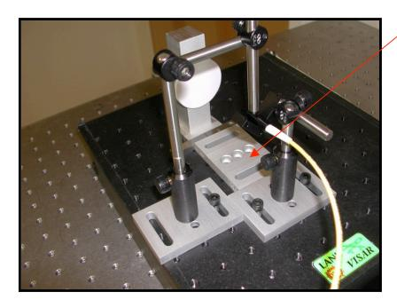
Spacers were 1mm wide to 9mm. The distance of the diffuser to the probe was varied from 1mm to 145mm.
