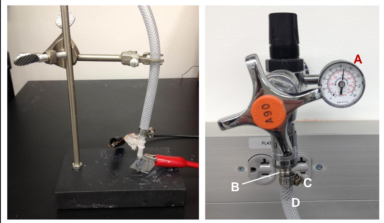
Compressed air at 85 psi is applied to the input reservoir and forces an ionic solution through the nanochannel or bank of nanochannels in the device. A pressure of 85 psi was selected to stay consistent with existing research in this field. The streaming potential, or voltage generated in the device, is measured across the channel. Data representing the relationship between pressure and potential will be presented in my defense.
