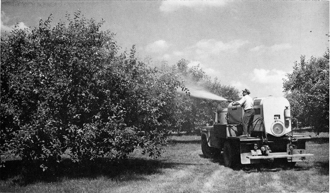
FIG. 1.—Hydraulic-pressure sprayer used to apply all dilute (1X) sprays.
