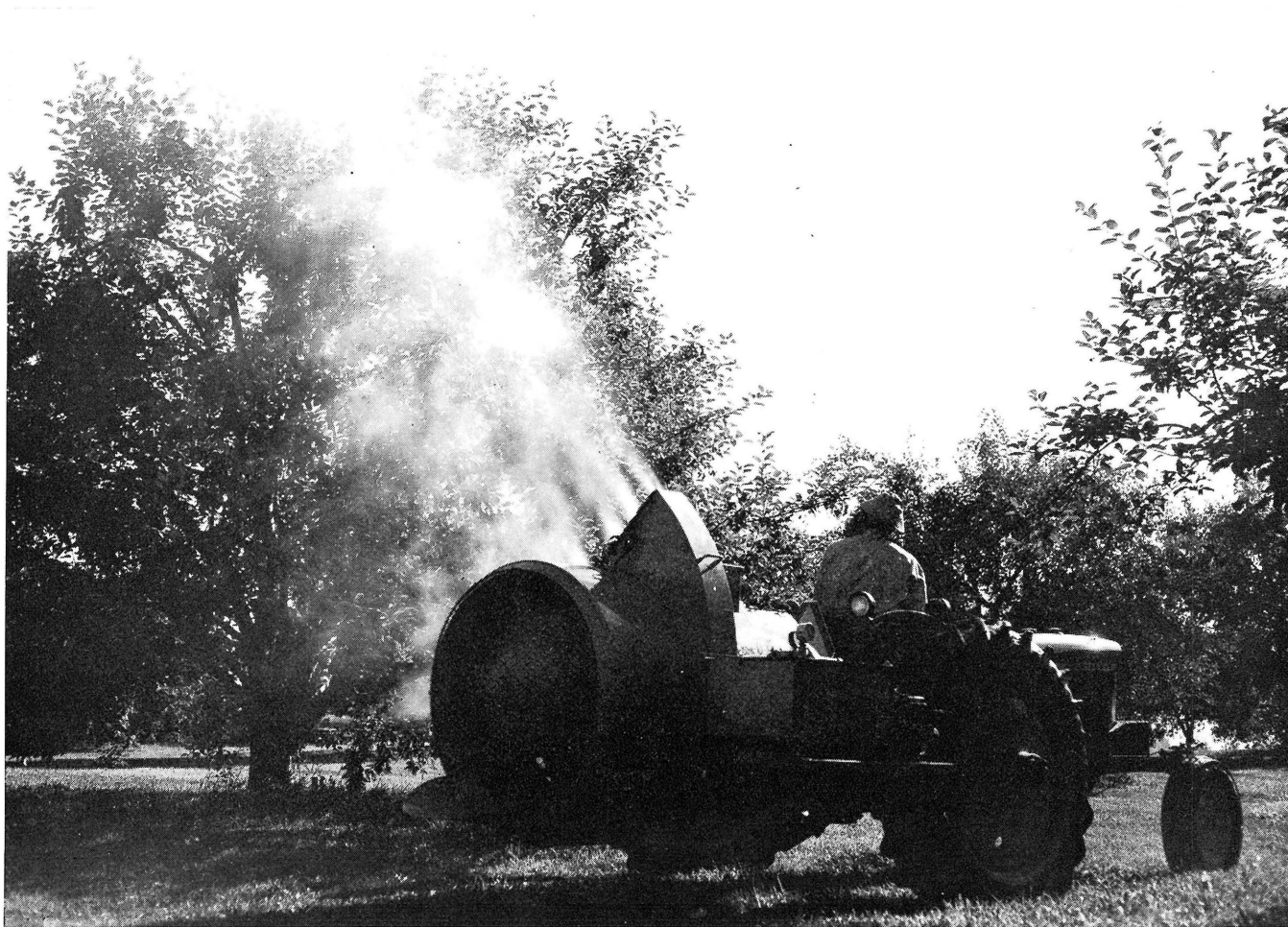
FIG. 3.—HC airblast sprayer used to apply 33X, 50X, and 66X sprays.
