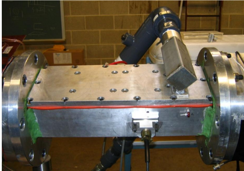
Figure 3: Test Section Containing Flat Plate
