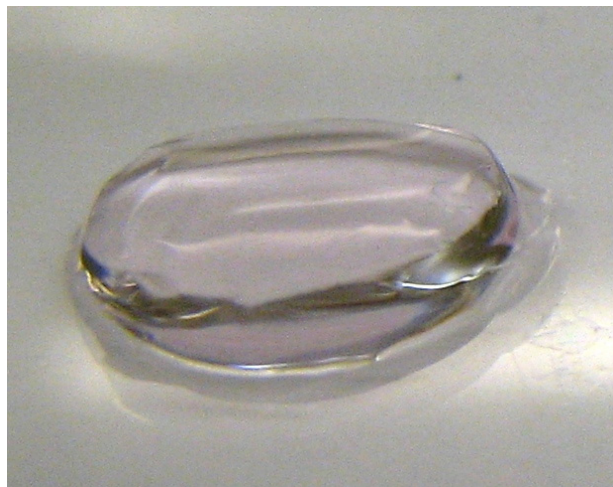
Figure 3.14: Composite Seaprep Agarose (1x) Hydrogel after 13 Days in PBS
