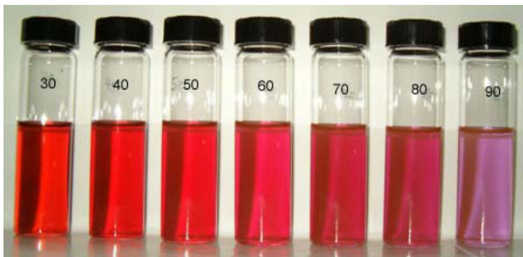
Figure 2.10: Dependence of Absorbance on Gold Nanoparticle Size (diameter – in nm) 13
