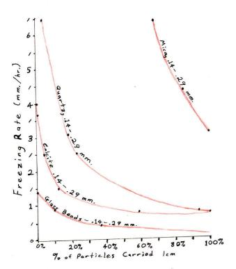
Fig. 1. Percentage, by weight, of glass beads, calcite, quartz, and mica which is carried 1 centimeter at varying rates of freezing. Illustrates the exclusion of particles by afreezing front. (Corte, 1963a)
