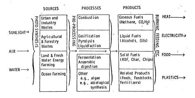
Figure 1. Biomass Sources, Processes, and Products.
