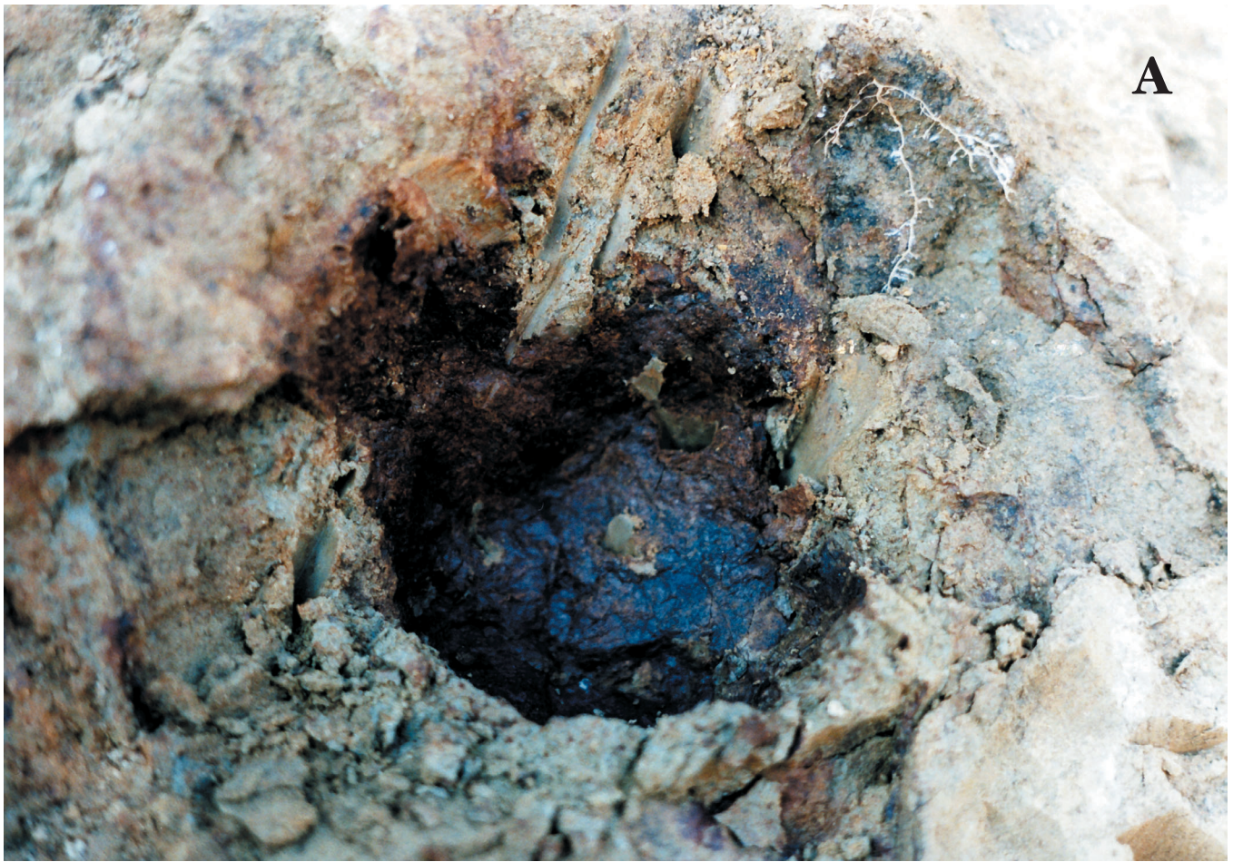
FIGURE 4. Ripped up “Clay Ball” clasts of Clermont lacustrine materials found at the Backbone Creek till cut, exhibiting the characteristic “green rust” colorations discovered in the borings around the CECOS site, next buried valley north. The unstable color of the matrix of the material was preserved in place from the time of deposition until they were discovered during a field investigation, Fall 1999. A characteristic yellowish-brown goethite color weathering rind forms around each section of the clay (Schwertmann 1993). Upon opening, the lacustrine matrix quickly oxidizes to the typical goethite colors. Photos by Julie Weatherington-Rice.
