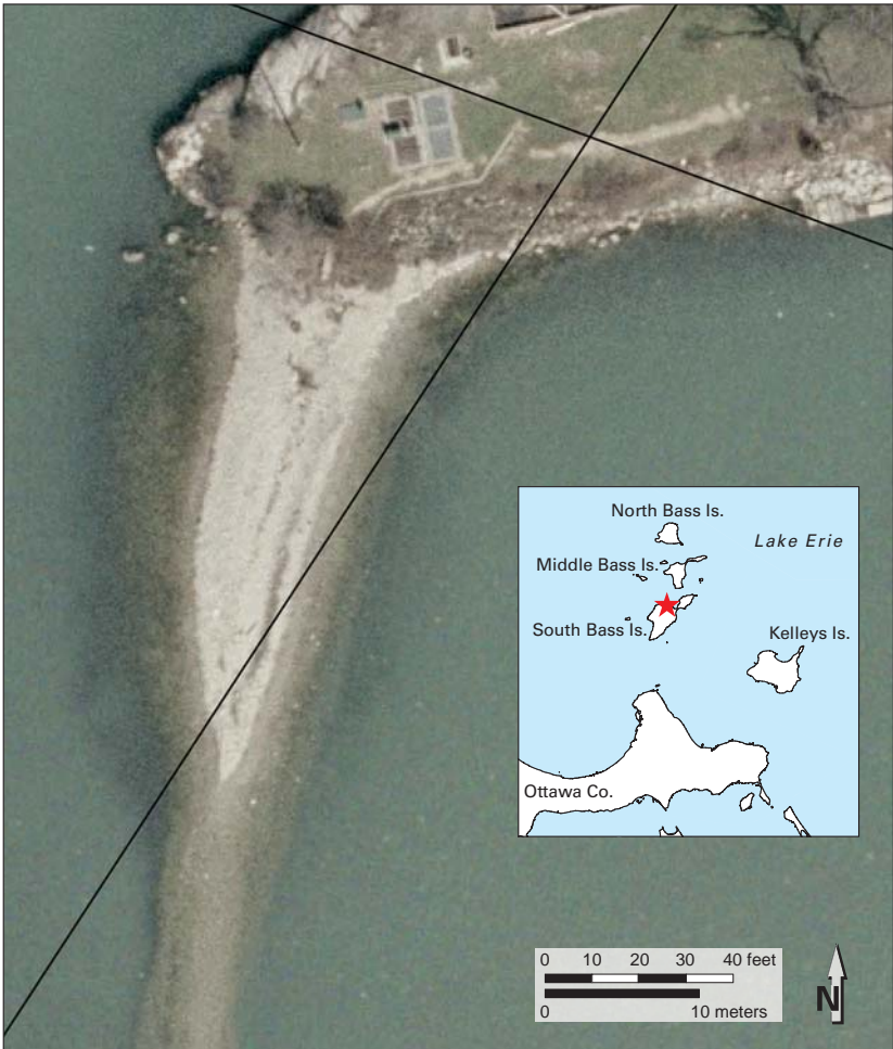
FIGURE 3.—Photo showing a Lake Erie Coastal Erosion Area transect that does not cross the beach in a meaningful way. Most such lines were established with a proper shoreline orientation, but later construction projects (in this case a jetty for a harbor) can render individual transects meaningless.
