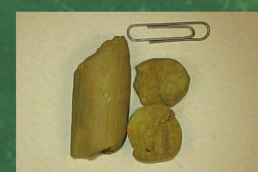
Figure 2: Sediment core from South Indian Run Cave; segment broken in half, with one half split again for alternate view.
