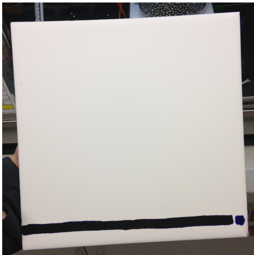
Figure 31: (VB)_2(CH_2)_2 run 4 (ACN) M&L prep TLC before developing, showing VB spotted on right side.
