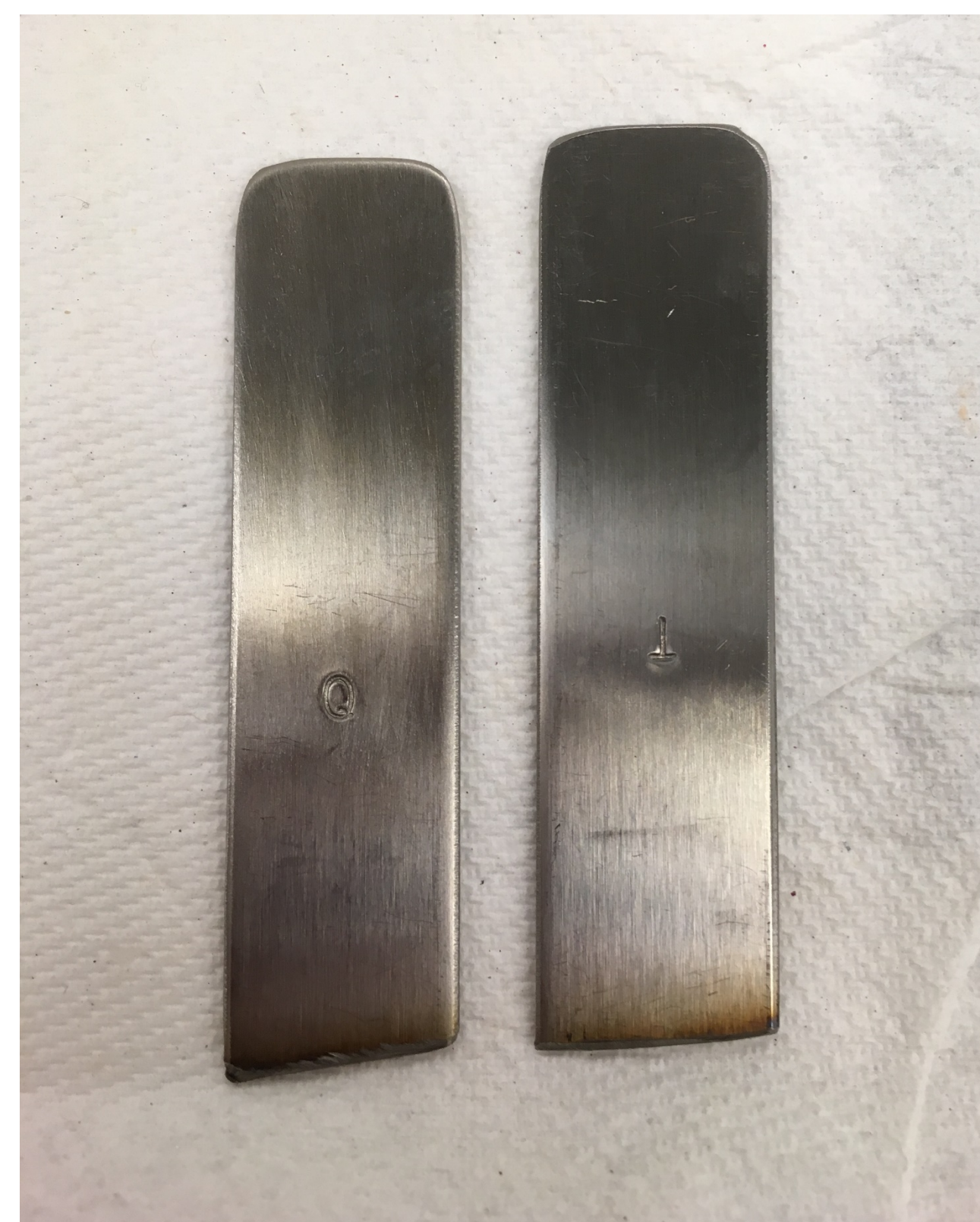
The roughest coupon, Q (pictured left) and the least rough coupon, T (pictured right).
