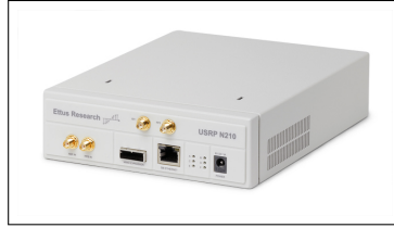
Figure 2.4: USRP N210 Software Defined Radio [11]
