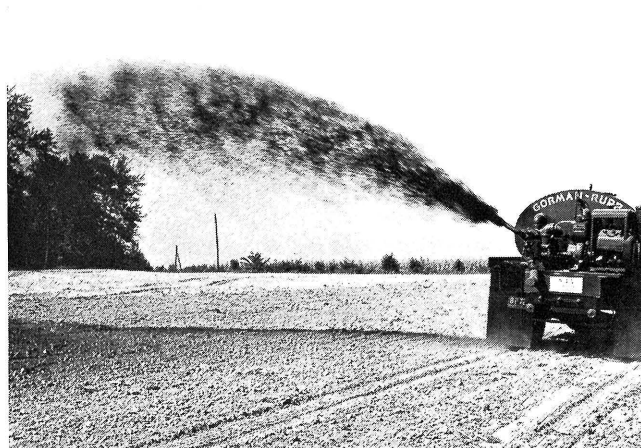
FIG. 7.—Commercial tank truck with pump discharge. Courtesy of Gorman-Rupp Co., Mansfield, Ohio.
