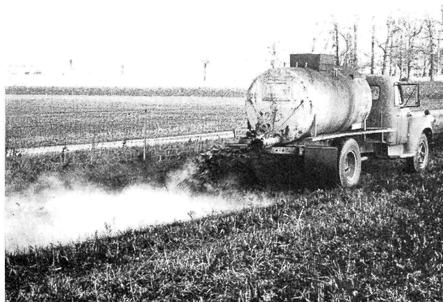
FIG. 13.—Spreading digested sludge on a cold day.
