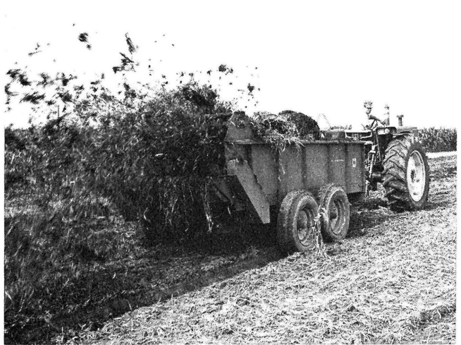
FIG. 5.—Conventional farm manure spreader.
