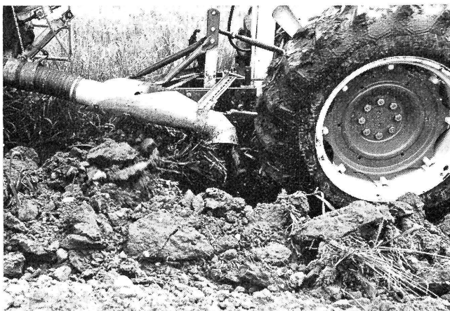
FIG. 8.—Covering of slurried waste with a single, moldboard plow. Courtesy of Prof. C. H. Reed, Biological and Agricultural Engineering, Rutgers Univ.
