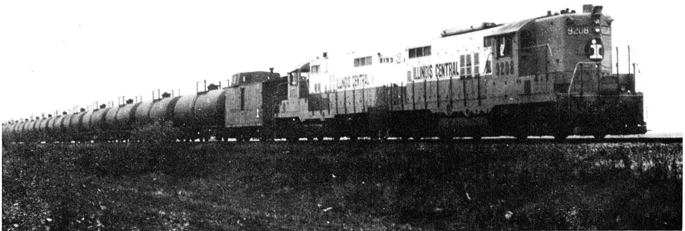
FIG. 2.—Rail tank cars used for hauling sludge from Chicago to Arcola, Ill.
