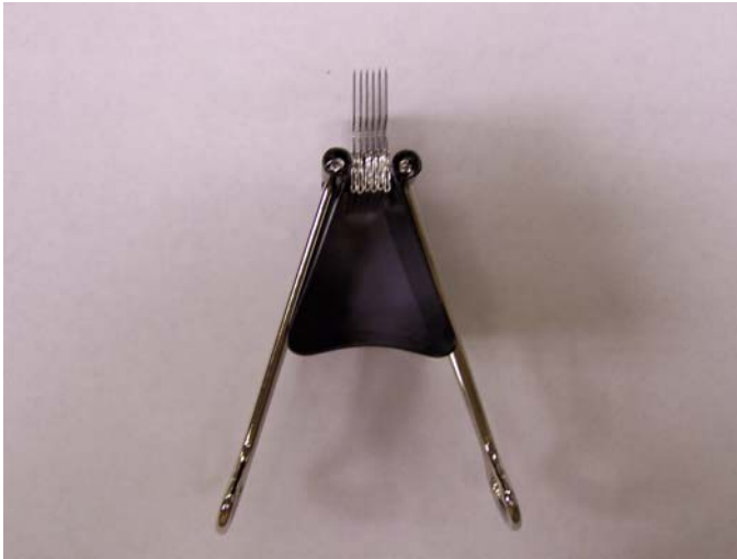
Figure 10. Binder clip with razor blades aligned for contamination with TMV and disinfectant treatments, Phase I.
