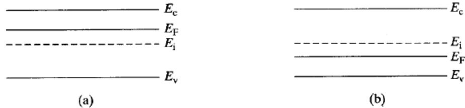
Figure 2: Diagrams of the energy band containing the intrinsic Fermi levels along with representations for a) an n-type semiconductor and b) a p-type semiconductor<sup>[10]</sup>
