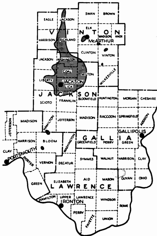
Figure 6. Generalized map of known major occurrences of minable Quakertown (No. 2) coal in Ohio.
