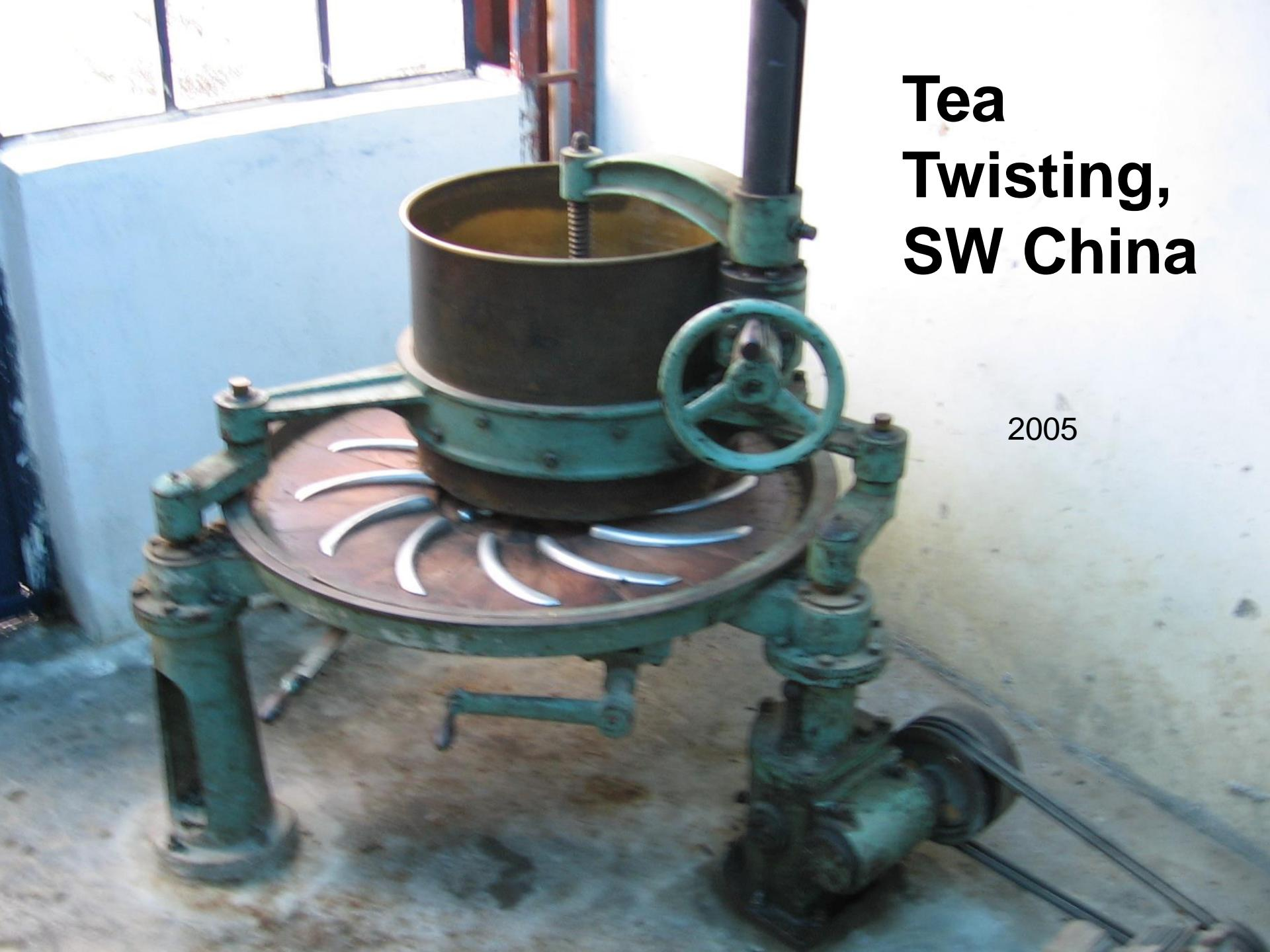
A vintage green tea twisting machine, featuring a large circular wooden base with a metal frame. The top assembly is made of dark wood and metal, with a prominent green painted metal wheel on the right side used for operating the machine. The machine is situated on a light-colored floor, with a window and some vertical poles visible in the background.
