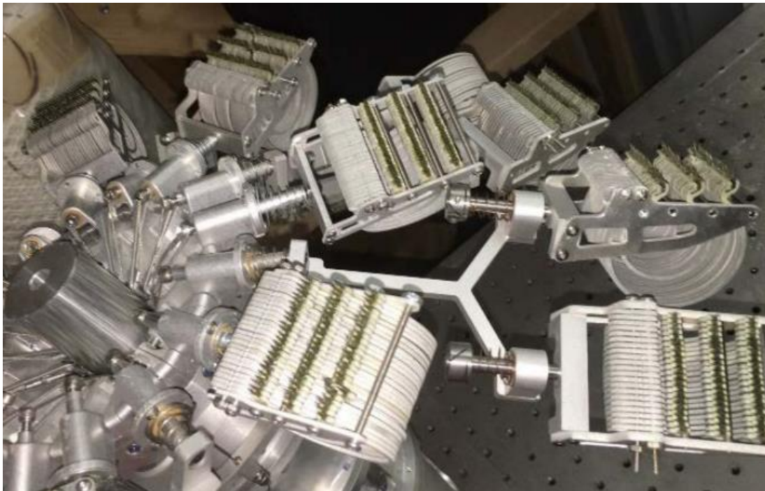
Figure 2: Microspines Arrayed into Multiple Carriages
