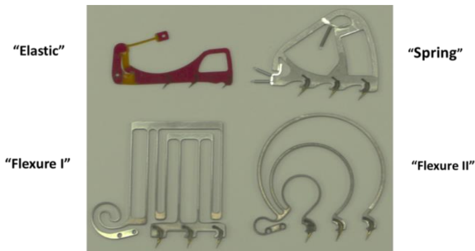
Figure 5: Examples of Previous Microspine Design Concepts
