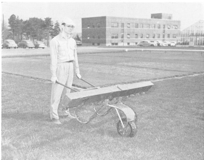
Fig. 1.—This is an experimental applicator made from the grass seed box of a drill.
