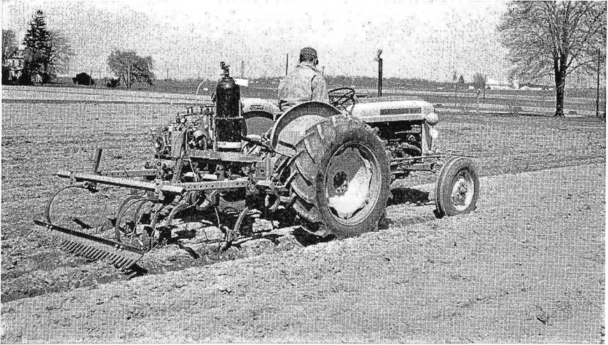
Fig. 5.—Type of specially designed applicator used to apply chloropicrin to the soil for nematode control.
