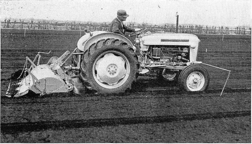
Fig. 3.—Type of rotary tiller used to apply SMDC and DBCP to muck soil and to prepare the soil in the untreated check and before the application of the other nematocides.
