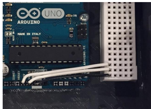
Figure 31: Creating the 3.3 Volt, 5 Volt, and Ground Buses on the Bare Breadboard
