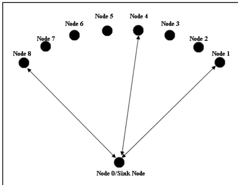
**Figure 1: “Desktop” Setup for Single-Hop Network Testing**
