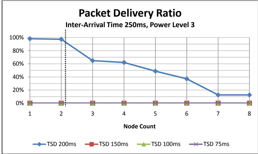
**Figure 23: Packet Delivery Ratio for Varying Timeslot Durations and Node Counts (Inter-arrival Time=250ms)**
