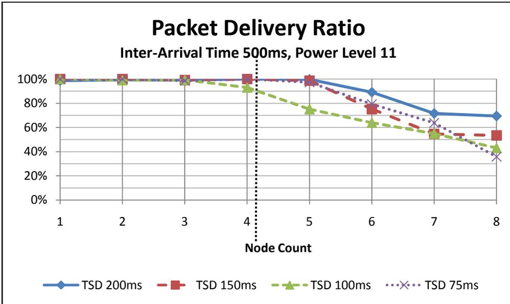
Figure 16: Packet Delivery Ratio for Varying Timeslot Durations and Node Counts (Inter-arrival Time=500ms)
