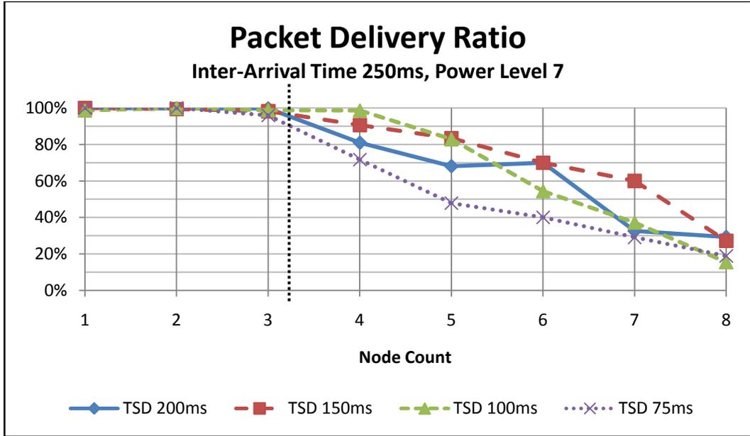
Figure 20: Packet Delivery Ratio for Varying Timeslot Durations and Node Counts (Inter-arrival Time=250ms)
