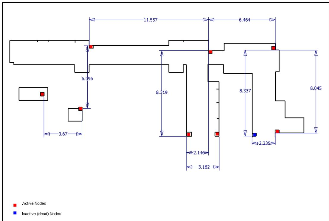
**Figure 2: Hallway Setup for Multi-Hop Network Testing**
