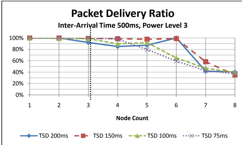
Figure 22: Packet Delivery Ratio for Varying Timeslot Durations and Node Counts (Inter-arrival Time=500ms)
