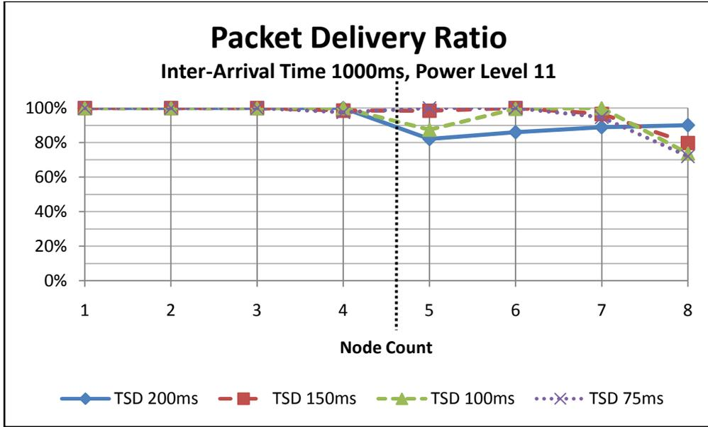
Figure 15: Packet Delivery Ratio for Varying Timeslot Durations and Node Counts (Inter-arrival Time=1000ms)
