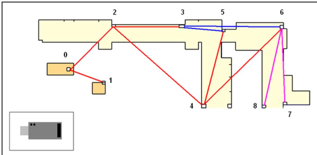
Figure 10: Network Topology for Horizontal Orientation, Antenna to Right
