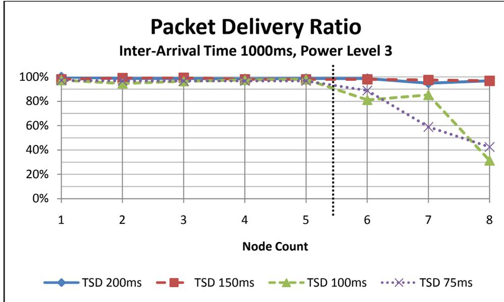
Figure 14: Packet Delivery Ratio with Constant Inter-arrival Time, Varying Power of Level 3
