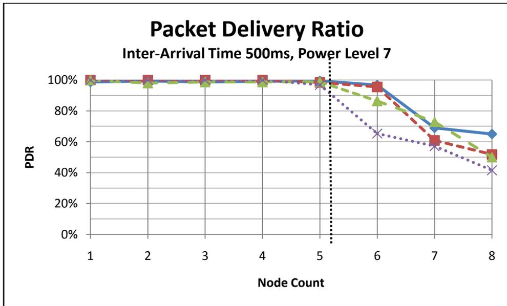
Figure 19: Packet Delivery Ratio for Varying Timeslot Durations and Node Counts (Inter-arrival Time=500ms)
