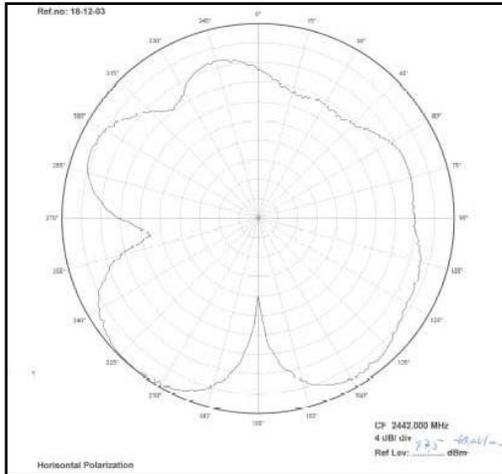
**Figure 4: Power Pattern for Horizontal Orientation [5]**
