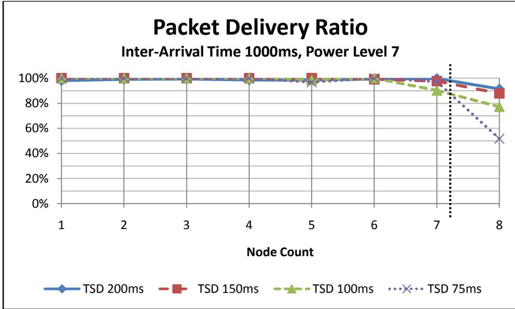
Figure 18: Packet Delivery Ratio for Varying Timeslot Durations and Node Counts (Inter-arrival Time=1000ms)
