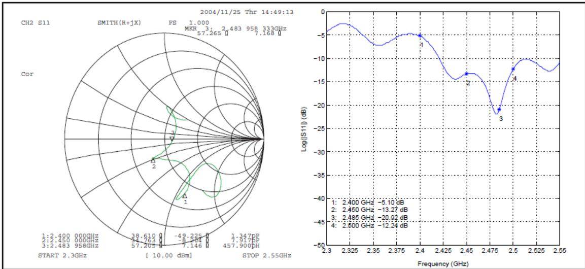
**Figure 6: VSWR for Module with Attached Battery Pack [5]**
