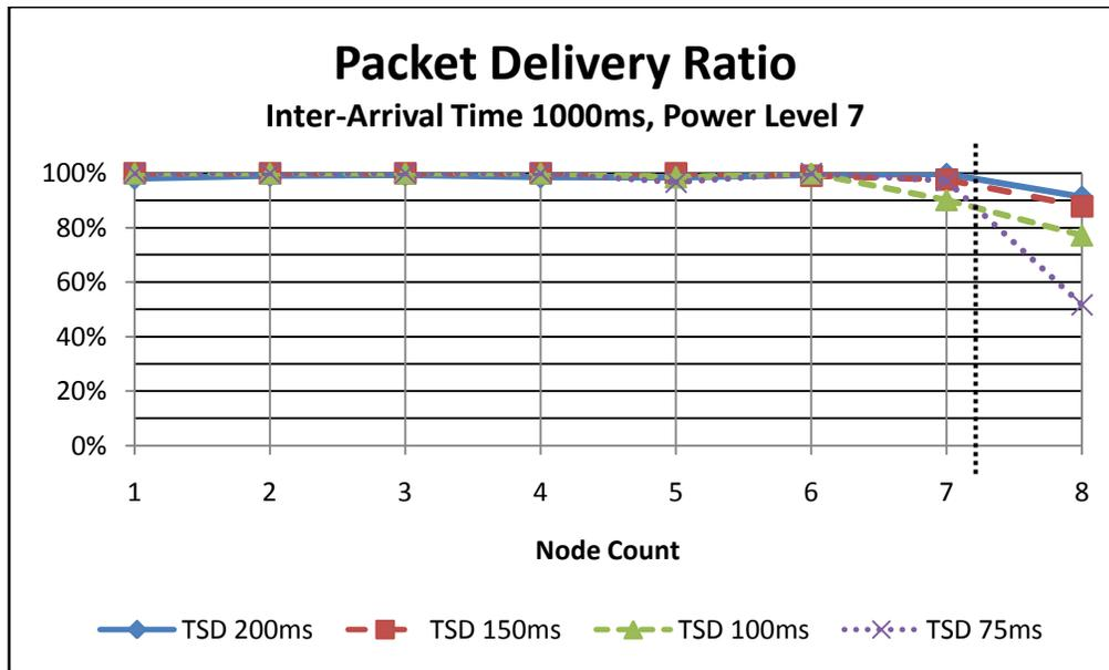
Figure 13: Packet Delivery Ratio with Constant Inter-arrival Time, Varying Power of Level 7
