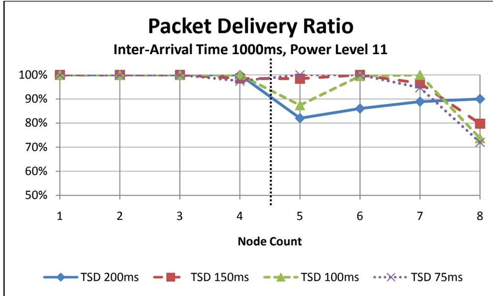
Figure 12: Packet Delivery Ratio with Constant Inter-arrival Time, Varying Power of Level 11
