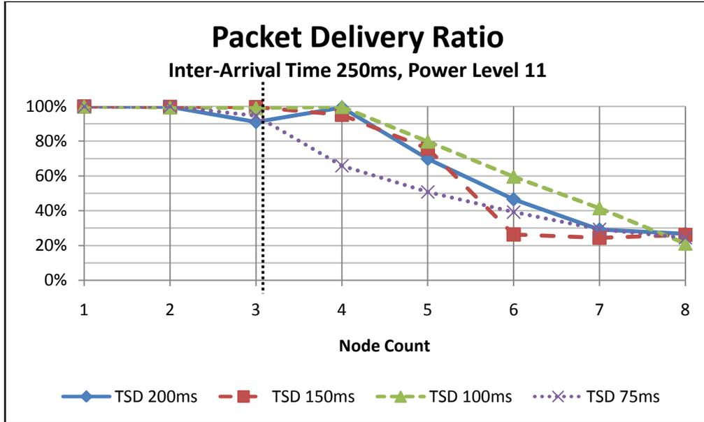
**Figure 17: Packet Delivery Ratio for Varying Timeslot Durations and Node Counts (Inter-arrival Time=250ms)**
