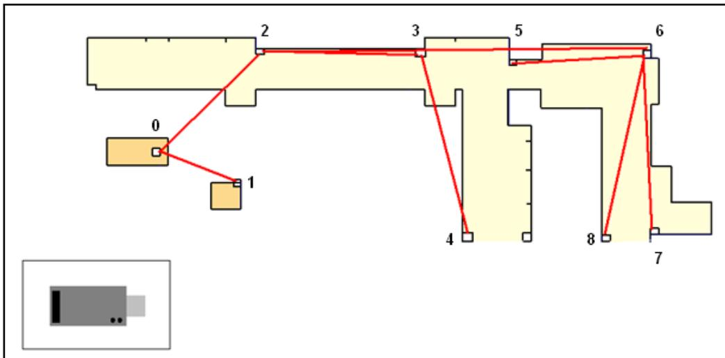
**Figure 9: Network Topology for Horizontal Orientation, Antenna to Left**
