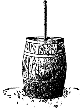
Fig. 2.—Arsenate of lead mixer A mixer for working up arsenate of lead paste. An old churn may be utilized; but if this is not available, a mixer may be made from a small keg. (From Ohio Agr. Exp. Sta. Bul. 232 (1909), p. 52)
