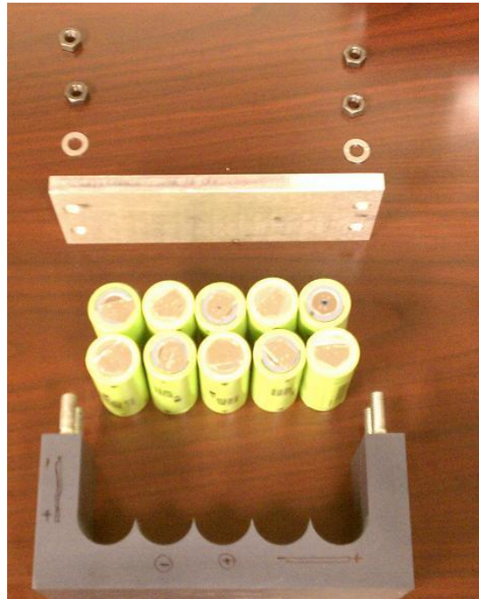
Figure 20: Components of new battery pack design
