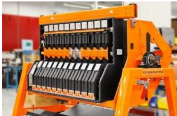
Figure 8: Liquid cooled Tesla Roadster Battery 4
