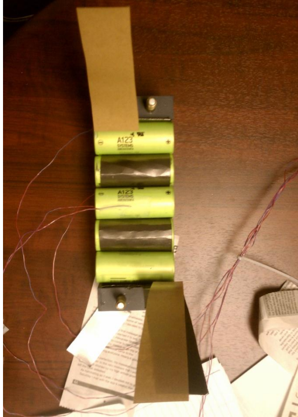
Figure 22: Top view of pack 2 prior to heat sink addition
