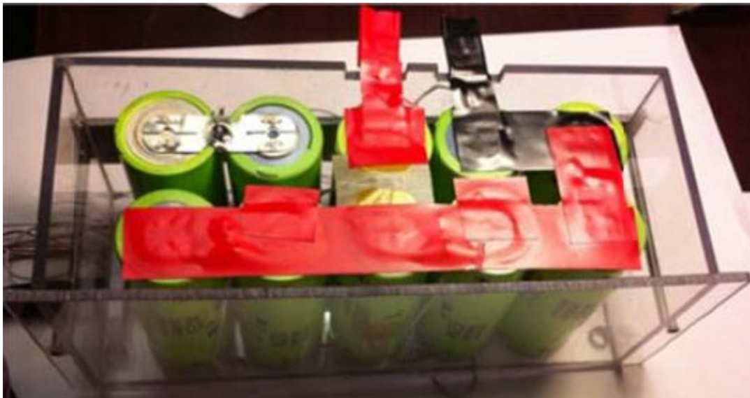
Figure 14: Battery pack configuration
