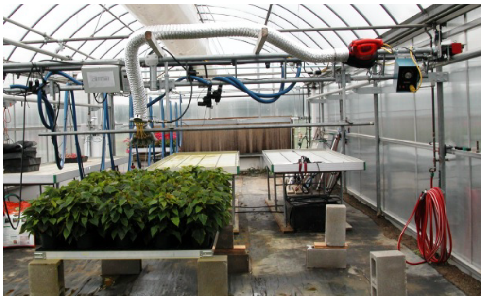
Figure 3. Watering boom with five-port, air-assist sprayer and blower.
