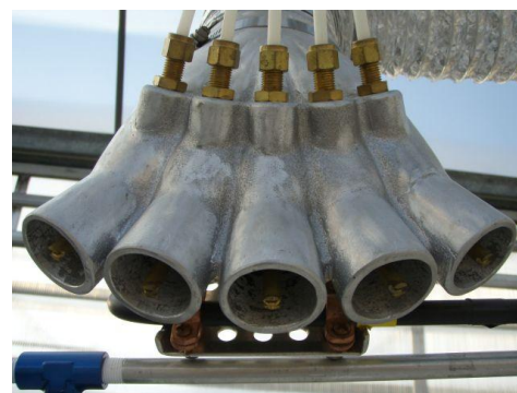
Figure 2. Five-port, air-assist sprayer manifold.
