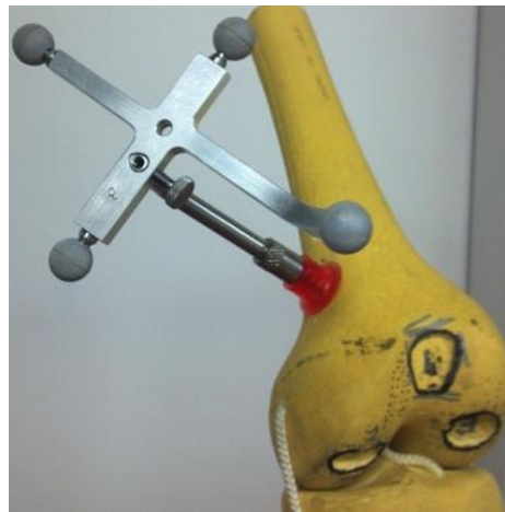
Figure 2.6: Attachment of optical tracker to bone utilizing the EZ-IO system.
