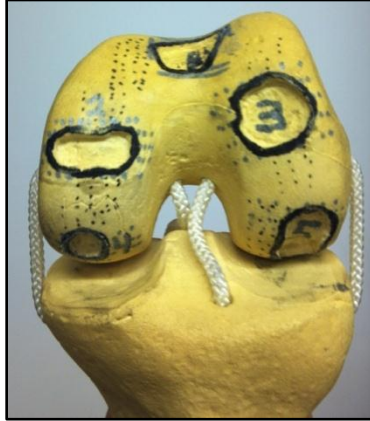
Figure 3.2: Artificial defects cut into Sawbones knee.
