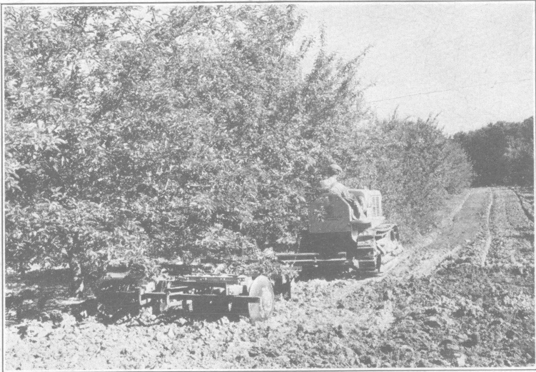
Fig. 8.—A disk with an extension hitch being used to cultivate an apple orchard
