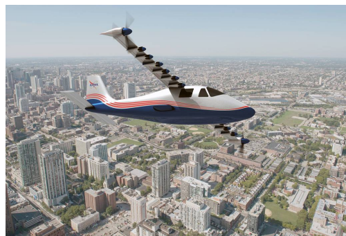
Figure 2: The NASA X-57 will demonstrate the benefits of distributed electric propulsion for fixed-wing aircraft [16]
