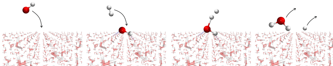
Figure 4.3 Eley–Rideal reaction mechanism. One particle is first adsorbed on a surface. A second one impinges from the gas phase and the products are directly formed.
