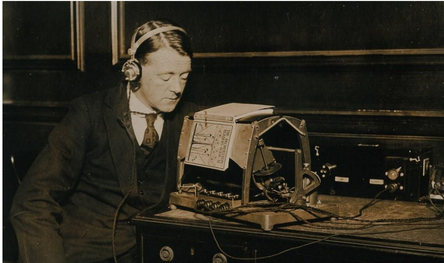
Fig. 3: Optophone for blind readers, patented by E. E. Fournier d'Albe. Device pictured here assembled by Barr & Stroud, ca. 1921. Credit: Wellcome Library, London and Wellcome Images, accession number PHO 4336.
