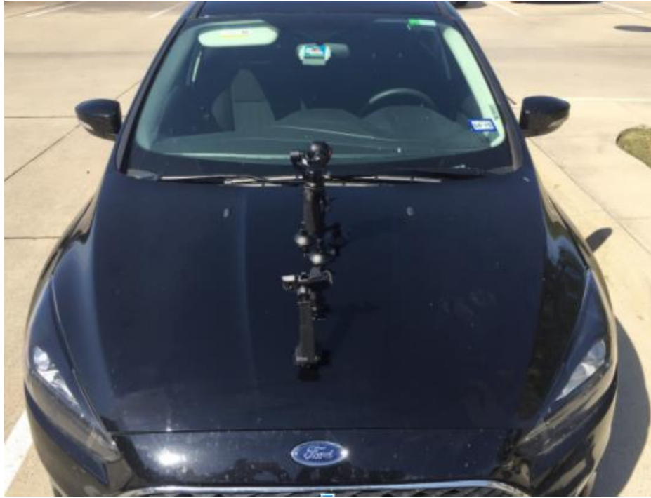
Figure 1. Positioning of the Osmo camera
