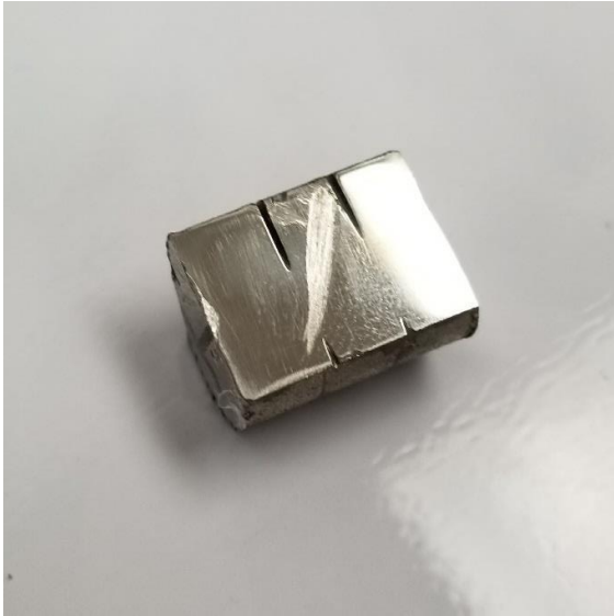
Figure 16. Cross section of three specimen before being separated, surface is polished and used for SEM Imaging.
