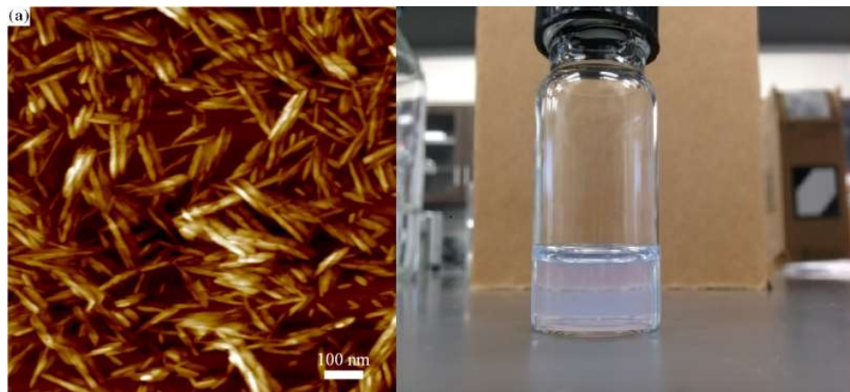
Figure 1: Left: AFM image of CNC, Right: 1 wt. % CNC suspension in DI water. [5]
