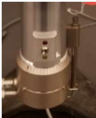
Figure 4: Cone and Plate with electronic gap setting function
