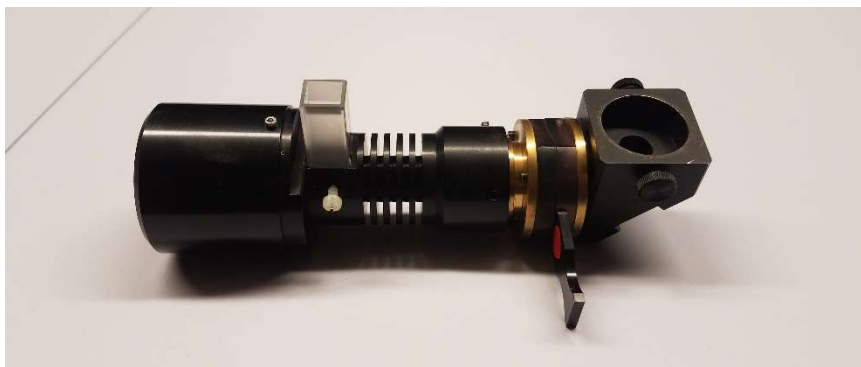
Figure 2.3.1: Photograph of Raman spectrometer cuvette holder
