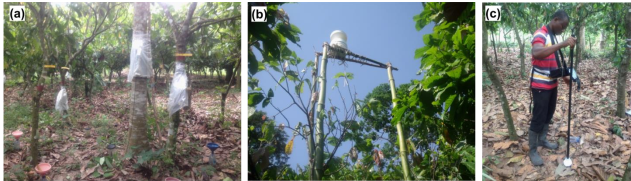
Fig.1 Pictures illustrate various measurements/devices employed to assess water dynamics in the investigated cocoa systems: (a) sap flux sensors installed on shade and cocoa trees protected with foil and plastic sheets and homemade rain gauges (bottom right) made of 14.5cm diameter funnels and 1liter plastic bottles, (b) tipping bucket rain gauge installed above cocoa canopy at a height of 6m and (c) soil water measurement with Diviner 2000 probe. The stick is introduced to pre-installed PVC tubes. Gravimetric water content can be read out every 10 cm down to 150 cm depth. The Diviner readings were calibrated against actual soil water content via soil sampling in dry and wet seasons.
