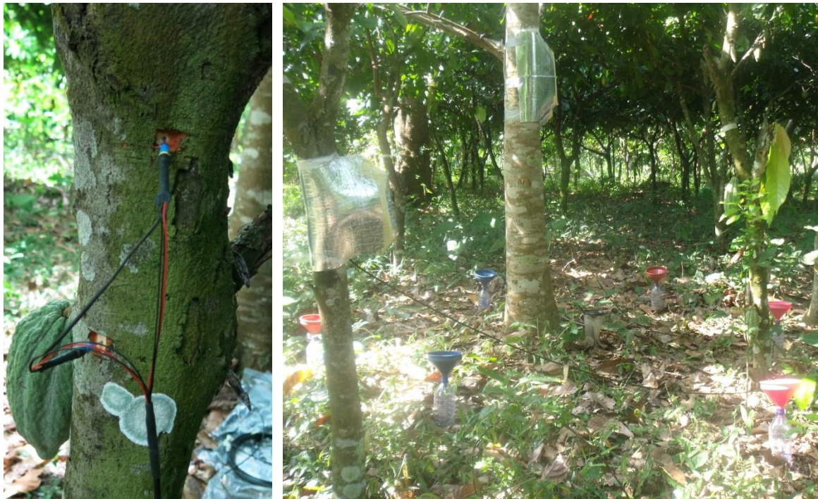
Fig. 8 Granier sap flux sensors installed on cocoa and shade trees
