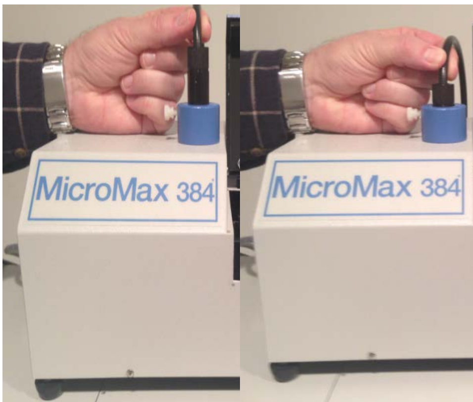
Figure 80: Positioning variance of fiber optic cable in MicroMax microwell plate reader. Photo courtesy of Lauren M. Ridley-Hoffman.
