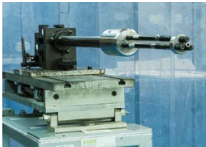
The image shows the RMA’s triple fragment launcher for testing PPE with near-simultaneous strikes. Image courtesy of Georgios Kechagiadakis and Marc Pirlot.
