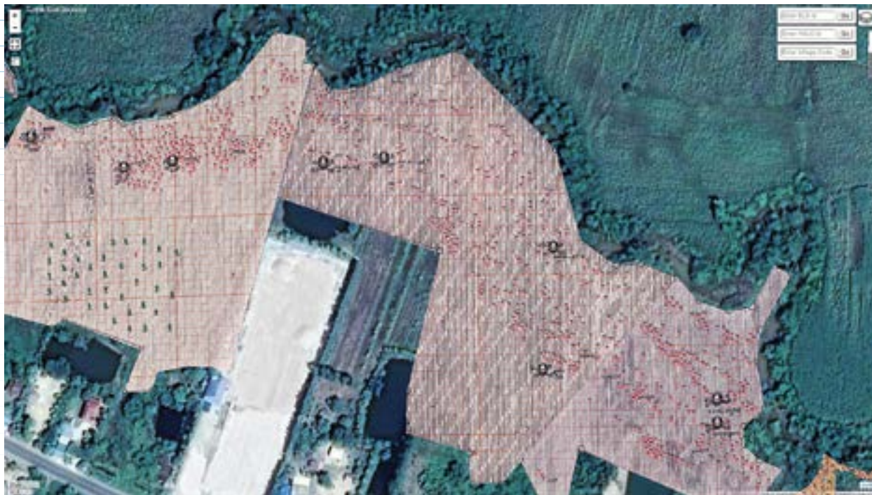
The same map with the mines and accidents digitized into HALO's PostgreSQL database and overlaid. All of this information is accessible via an ArcGIS Server web service on an interactive web map to operations staff.
