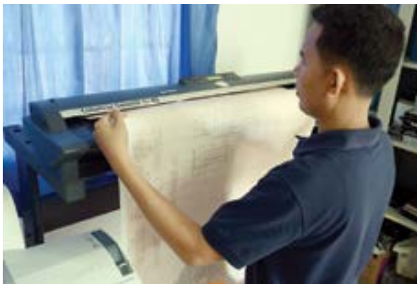
A data clerk scans a minefield sketch map from the field using a Colortac SmartLF Ci 40 large-format scanner and georeferenced it on top of minefield polygons in GIS.
