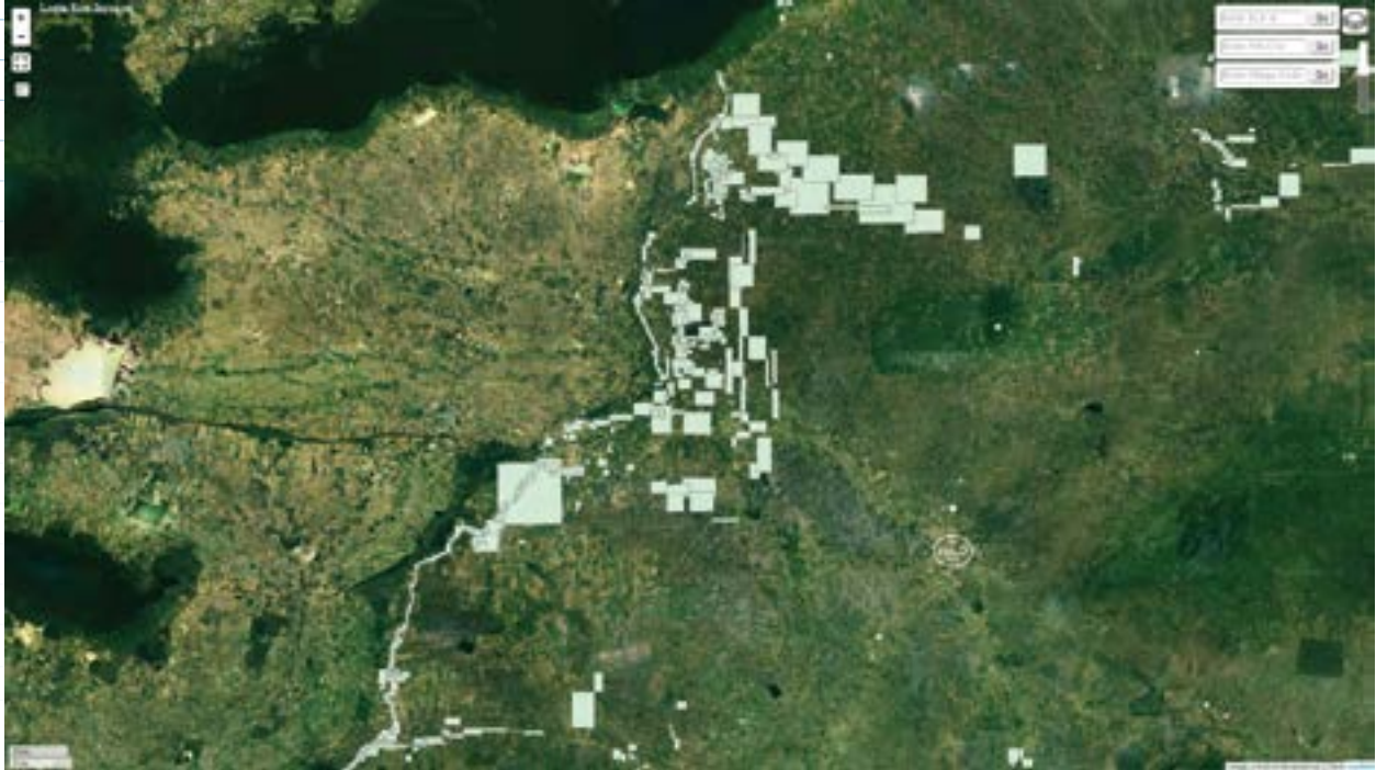
Boundaries of sketch maps georeferenced in GIS creating a nationwide mosaic and displayed in a web map. The sketches display once zoomed in on the web map.
