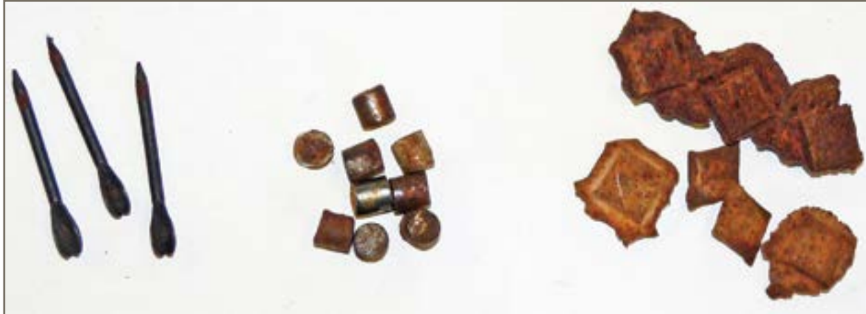
Left to right, the image shows flechettes from a munition, pre-chopped fragments from a bounding fragmentation mine, and pre-scored diamond fragmentation from a submunition. Image courtesy of the author.
