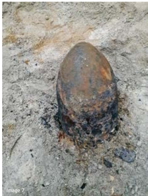
A 500 lb U.S. General Purpose (GP) bomb subsequently excavated at this site. The target was reflected off of bedrock, resulting in a nose-up orientation that prevented triggering of the delayed-action fuse.
